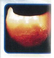
The residue from combustion at the end of the hearth is referred to as clinker. This is extracted from the furnace by a drum, then cooled and extinguished in an extractor unit. It is then evacuated using conveyor belts, with ferrous residue being removed using a magnetic separator. The clinker is then stored in a pit and removed by road transport.
